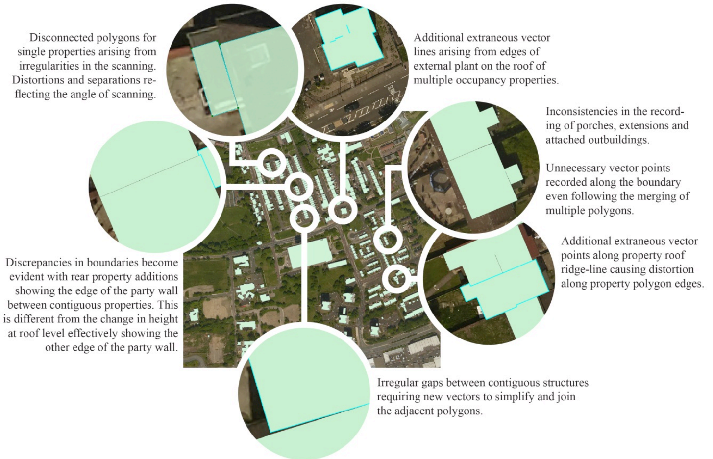
Fig 2: Highlighting the initial LiDAR data errors.
